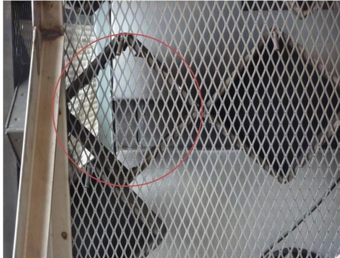
Figure 4: Failure of an arc test – highlighted indicator burned completely
