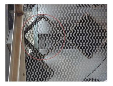
Figure 4: Failure of an arc test – highlighted indicator burned completely
