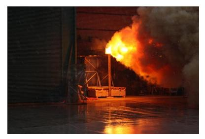
Figure 5: A Successful Arc Test of Vesta
