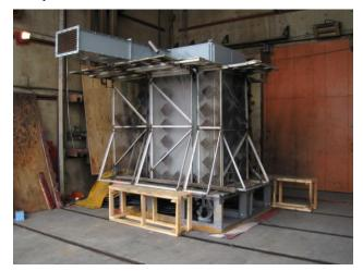
Figure 3: Vesta Switchgear set up for Arc Test at KEMA, Chalfont, PA
